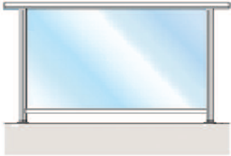
Figure 7 Fully framed infill panel
